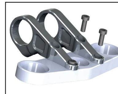
**Step 3:** Mount the 2 stem-halves on the upper fork crown. Attach screws only finger tight – make sure that the bottom surfaces of the stem attach properly to the upper fork crown.
