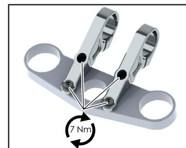
**Step 5:** Now tighten the 2 stem-halves on the upper fork arch via the 4 M6-screws, each at 7 Nm.
