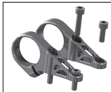
**Step 3:** Mount the 2 stem-halves on the upper fork crown. Attach screws only finger tight – make sure that the bottom surfaces of the stem attach properly to the upper fork crown. There are 2 screw lengths to be used – the longer ones (M6x25) need to be used in front 2 sunken holes / upper fork crown that are closer to the handlebar, the shorter ones (M6x16) attach at the backside as shown.
