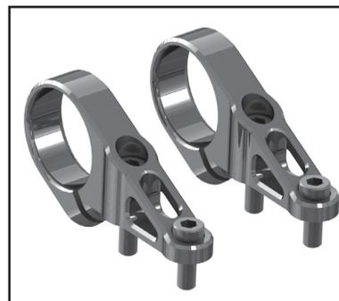
**Step 5:** Now tighten the 2 stem-halves on the upper fork arch via the 4 M6-screws, each at **7 Nm**.
