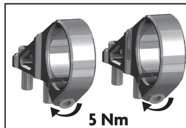
**Step 4:** Make sure that the assembly is not under tension – now align your handlebar to the desired angle / position and tighten it at a torque of **5 Nm**.
