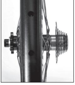
Then you are free to combine your transmission ratio. Between the following cogs, use the standard spacers (C), only the smallest 2 need always to be run spacerless.
