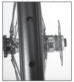
If you intend to run 7-speed on a standard hyperglide-freehub, you always need to place the wide spacer where it is written "7-speed" first on the freehub.
