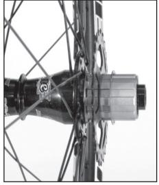
In this combination, simply start with the 25-teeth-cog on the freehub body
